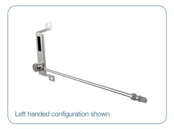
The Spec Master range of header rail assemblies are designed for use with non-corrosive or toxic, high purity gases up to grade 6.0 purity (99.999%). They are produced from nickel plated brass barstock and cupro-nickel tube and are intended for use in conjunction with our gas control panels integrated within gas management and distribution systems
